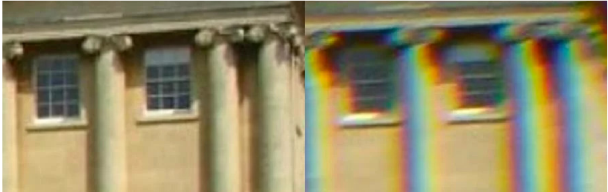
Figure 2.9: Example of lens distortion and chromatic aberration [23]
