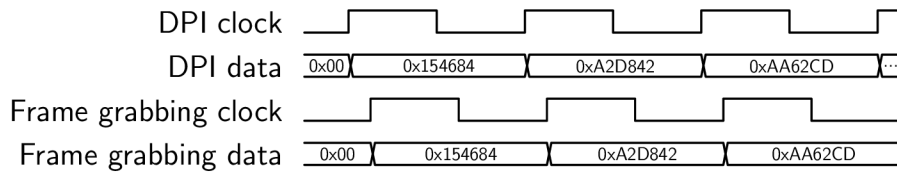
Figure 2.12: Theoretical timing diagram of frame grabbing hardware [source: author]
