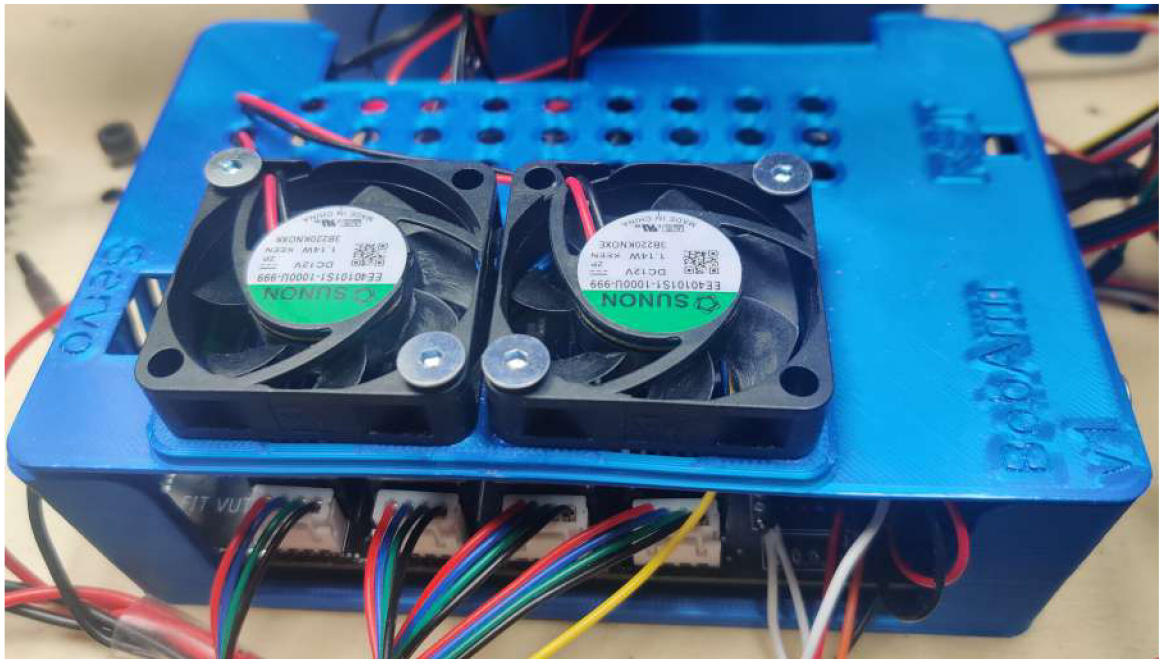
Figure C.1: The covering box for main control board
