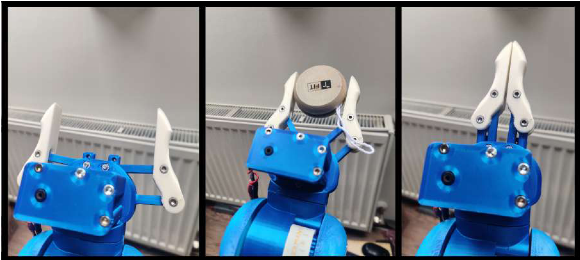
Figure 5.14: Visualization of gripper state (fully opened, closed with an object, fully closed)
