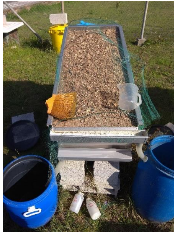
FIGURE 4 LYSIMETER BOX WITH FOREST CONTROL SOIL. GUTTERS CONNECTED BY TUBES TO COLLECTION TANKS ARE VISIBLE (TANKS HERE WITHOUT LIDS). ON THE GROUND, ONE BOTTLE WITH A WATER SAMPLE FROM EACH TANK. SEPTEMBER OF 2020
