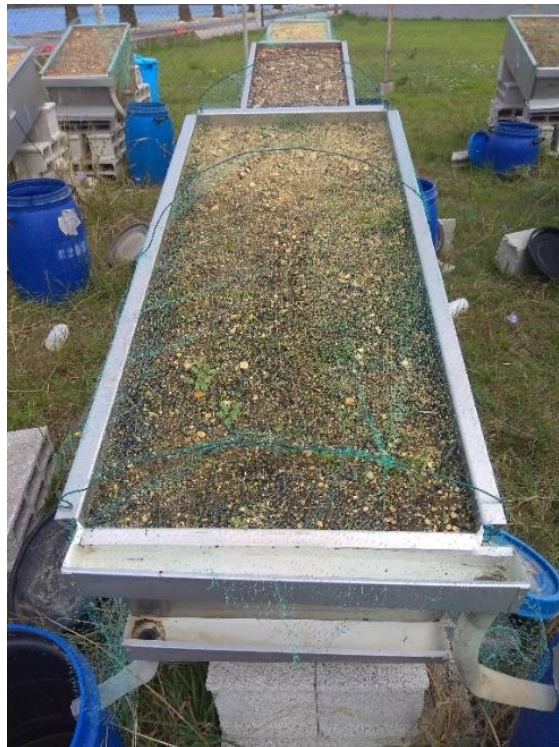
FIGURE 7. LYSIMETER WITH GROWING VEGETATION, COVERED WITH NET TO AVOID BIRD'S INTRUSION.
