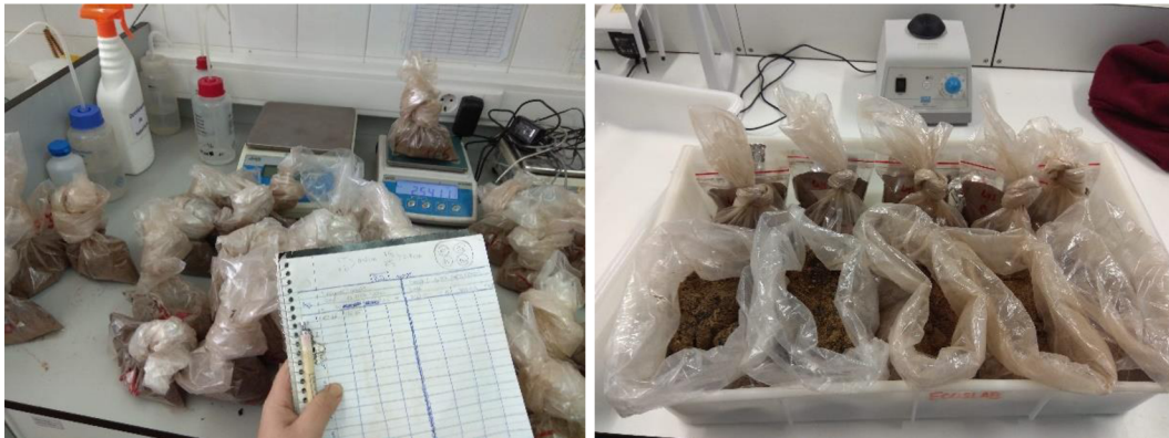
FIGURE 11. SAMPLES WEIGHTING AND PREPARED FOR OVEN-DRYING IN THERMAL BAGS.
