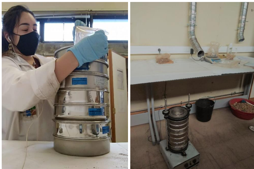
FIGURE 10. SETTING SAMPLES INTO SIEVING LAYERS FOR SIEVING MACHINE
