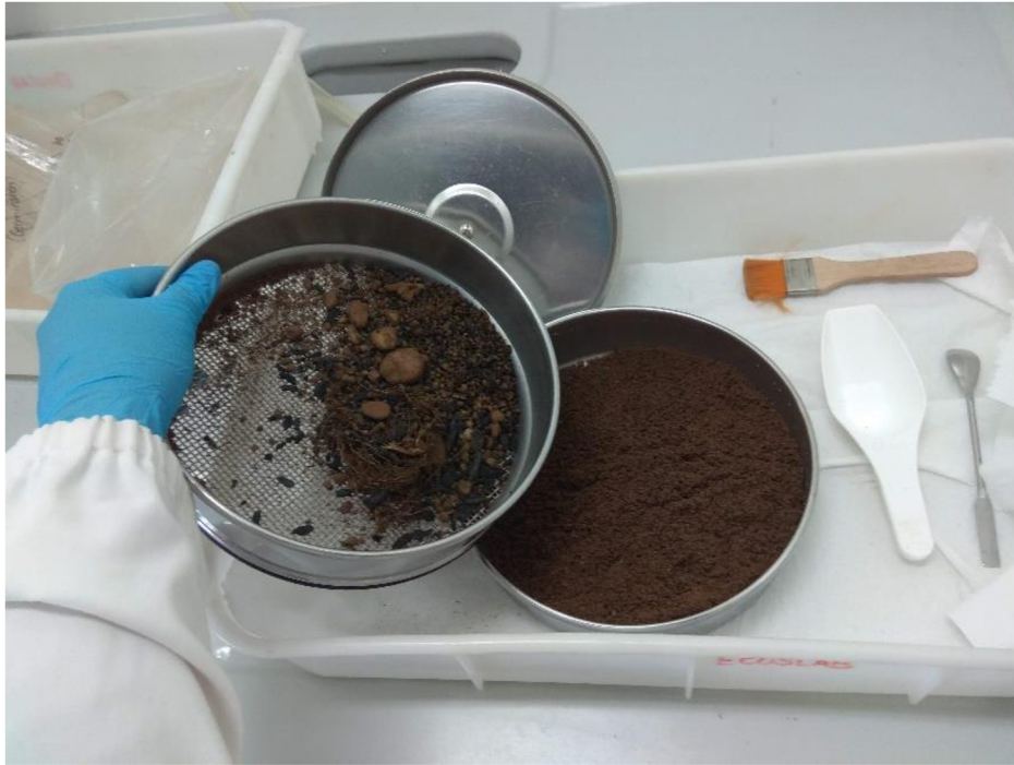
Figure 8. Sieving by hand with a 2 mm diameter sieve layer.
