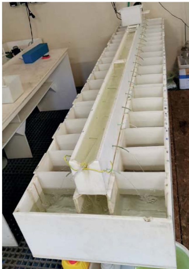
Fig. 4. Experimental incubation tank with 300 L re-circulated water and small boxes into which Petri dishes containing sterlet eggs were placed and incubated at 17 °C.
