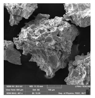
Figure 39: Eroded particles, source: CEITEC
