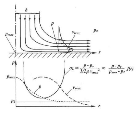
In Figure 11, a dependency of pressure, velocity and local cavitation number on radius is displayed.
