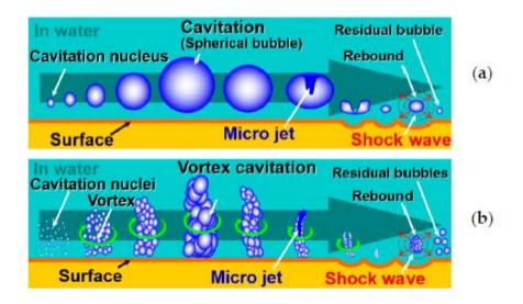
Figure 6: Cavitation inception, growth and collapse in case of spherical bubble (a) and vortex cavitation (b) [13]
