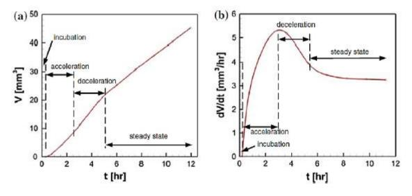
Figure 23: Cumulative volume loss (a), rate of volume loss (b) [2]
