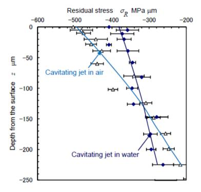
Figure 12: Compressive residual stresses [25]
