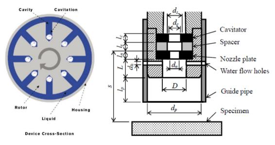
Figure 21: Cavitator (left) [29], nozzle with water flow holes (right) [30]
