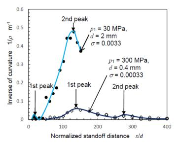
Figure 14: Dependency of cavitating jet aggressiveness (inverse of curvature radius) on the standoff distance [25]
