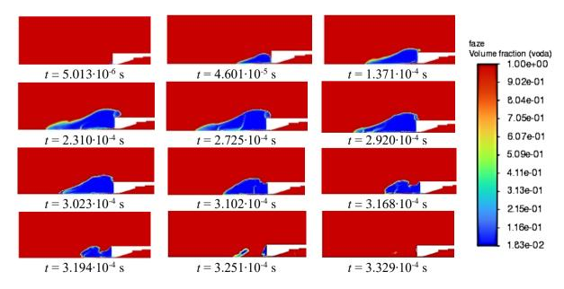
Figure 56: Set of images of volume fraction (water) - computation no. 5
