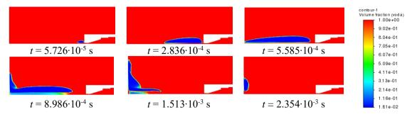
Figure 58: Set of images of volume fraction (water) – computation no. 6
