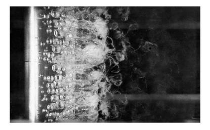
Figure 1: Formation of cavitation [5]
