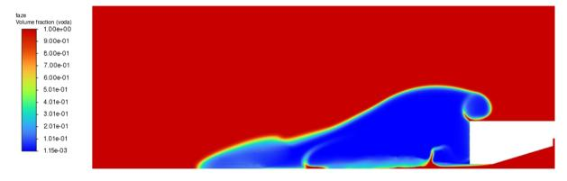
*Figure 57: Detail of the cavitation cloud at time*  $t = 2.582 \cdot 10^{-4} s$
