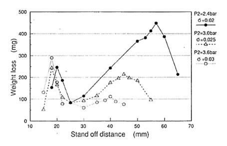
Figure 13: Weight loss dependent on the standoff distance [13]
