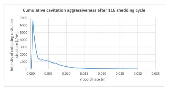
Figure 66: Cumulative cavitation aggressiveness after approximately 116 shedding cycles
