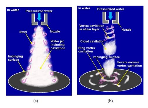
*Figure 10: Cavitation damage induced by swirl (a) – incorrect, damage created by ring vortex cavitation (b) – correct [13]*
