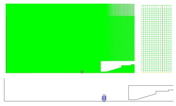
Figure 62: Monitoring area (dark red line  $-h_{agr}$ ) and one of the 4 monitoring points (left), detail of the grid with  $h_{agr}$  (right), locations of all the monitoring points (bottom)
