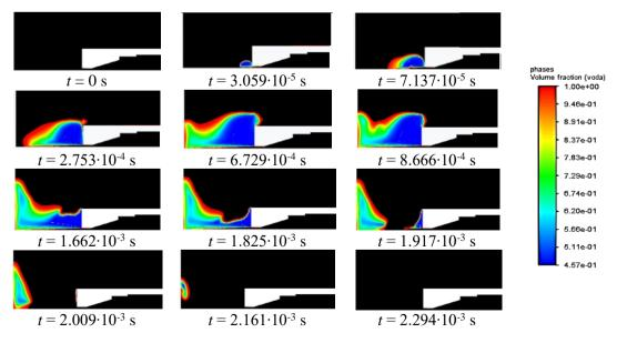
*Figure 52: Inception, growth and decay of the cavitation – computation no. 1*
