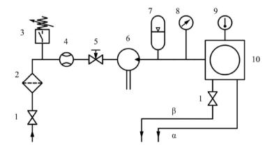
*Figure 28: The whole testing circuit - (1) shut-off valve, (2) filter, (3) pressure switch, (4) flowmeter, (5) control valve, (6) pump, (7) hydraulic accumulator, (8) pressure gauge, (9) thermometer and (10) test chamber [31]*
