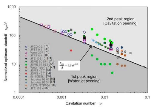
Figure 15: Classification map for cavitation erosion and water jet cutting [25]
