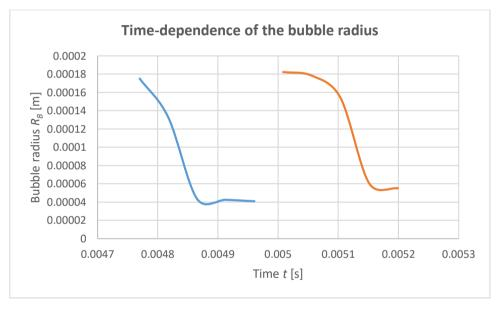
Figure 64: Bubble radius throughout two shedding cycles
