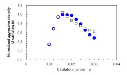
Figure 19: Normalized cavitation intensity as a function of cavitation number; blue dots correspond to the experiment, the white squares were obtained from following equations [13]
