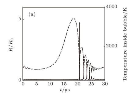
Figure 4: Cavitation bubble collapse and its rebounds [9]
