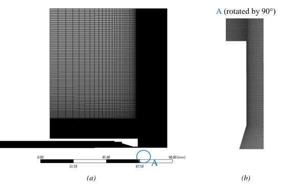
Figure 46: The coarse mesh (a) and its detail in the nozzle throat (b)
