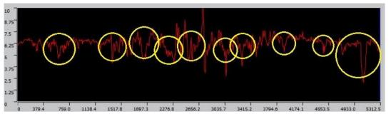
Figure 43: Profilometry of the pit region, source: CEITEC
