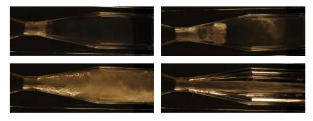
Figure 2: Stages of cavitation in Venturi tube - inception (upper left), growth (upper right and bottom left), supercavitation (bottom right) [6]
