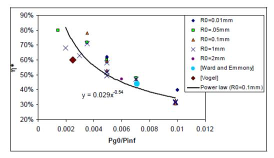
Figure 61: Collapse efficiency [41]
