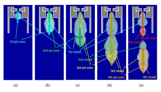
Figure 9: Development of cavitating jet [13]
