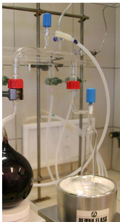
Fig. 32 Removing solvent under vacuum.
