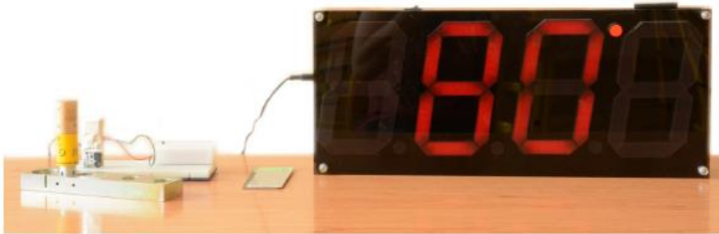
Figure 5. Set-up for absorption coefficient measurements.
