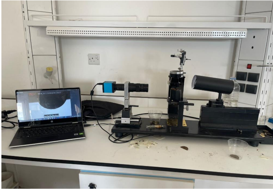
Figure 14 The VIT-6000 apparatus employed to measure CA and IFT.
