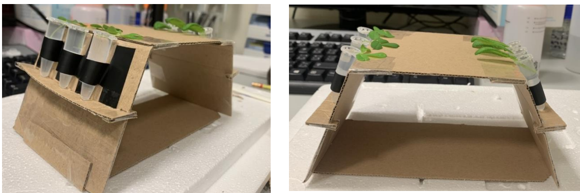
Figure 12. Cardboard stand with Eppendorf tubes (1,5 ml) filled with water used for capturing the exact moment of drying. There are small holders under the tubes that were taken away during the measurement and the tubes could move downwards.
