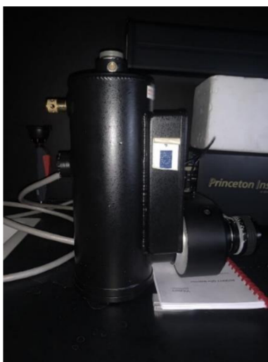
Figure 11. The CCD camera VersArray 1300B with a container for liquid nitrogen placed in the dark room.
