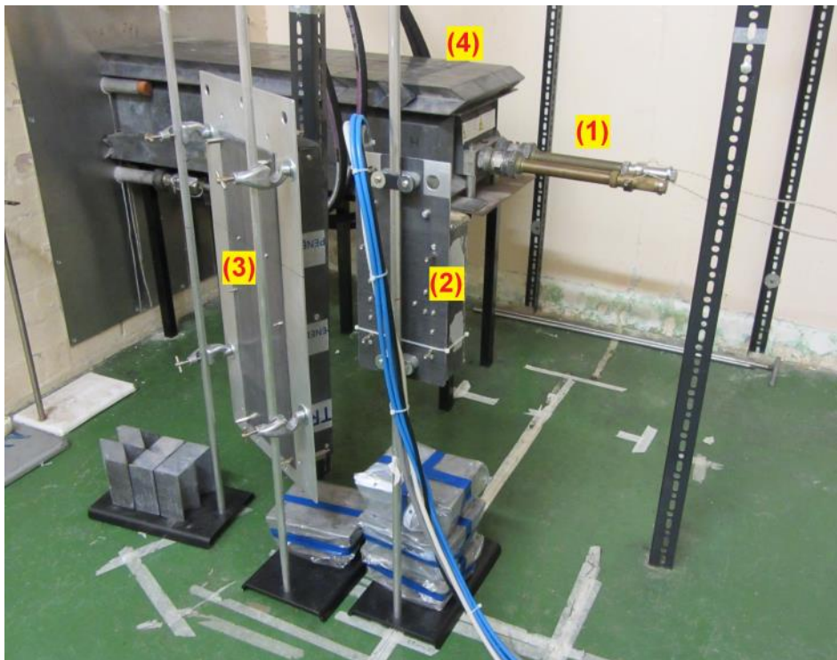
Fig. 6.1: A view of the irradiation area of the MIF during a PhD experiment. Two irradiation containers (2), (3) were placed in front of the sources (1). The source shielding block (4) allows for short irradiations (it reduces the travel time during which the sources are exposed).
