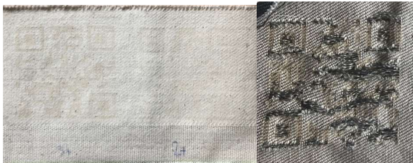
Figure 23: Washed out samples (X2 material) and damaged sample X1
