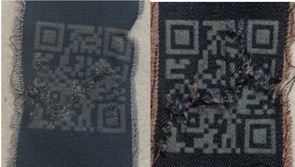
Figure 54: Breaking of engraving in patches.
