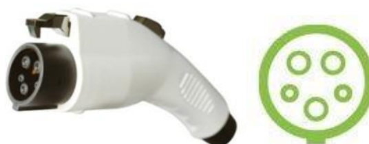
obr. 21 Konektor Typ 1, SAE J1772, Yazaki (Jet Charge 2017; The Mobility House 2017)
