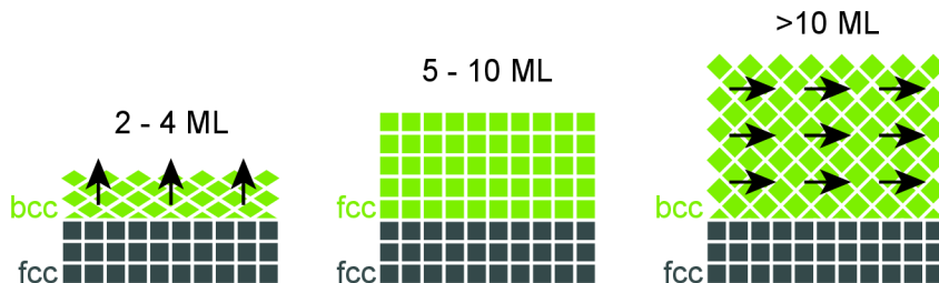
Fig. 2.2: Schematics of Fe/Cu(100) crystal structure, modified from [114]. The first schematic illustrates the earliest stage of growth – the ferromagnetic nanomartensitic structure, the second depicts the pseudomorphic growth of the paramagnetic fcc structure, and the third one depicts growth of the ferromagnetic bcc structure after releasing strain in the Fe layer. In both ferromagnetic growth regimes, preferred orientation of the magnetization vector is indicated by black arrows.
