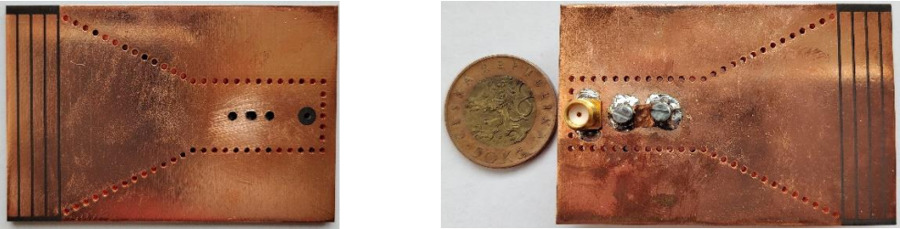
Fig. 6.4 a) Fabricated antenna b) Antenna with tuning pins and SMA connector
