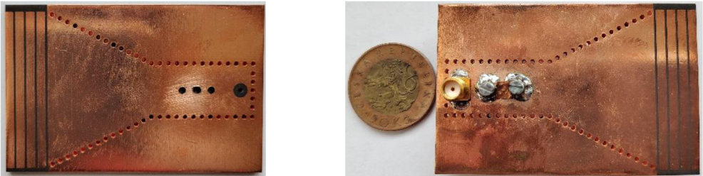
Fig. 6.4 a) Fabricated antenna b) Antenna with tuning pins and SMA connector
