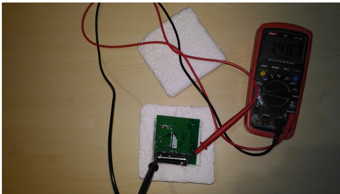
Fig. G.7: Femtostrat-1 post-flight voltage check - Credit: Marián Lukačko
