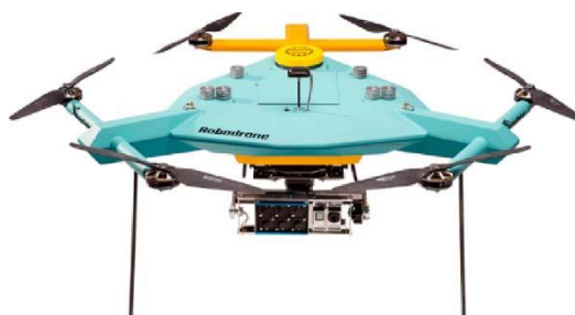
Figure 2. UAV Robodrone Kingfisher with a mounted multispectral camera Tetracam Micro-MCA6.
