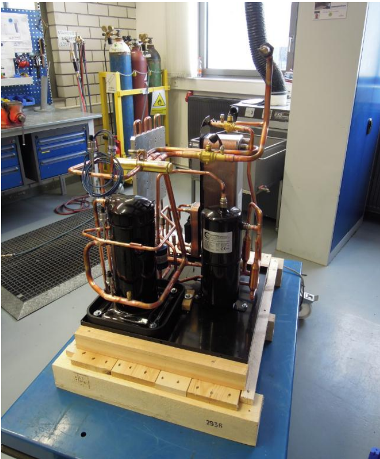
Fig 4.2 and 4.3.: Heat pump during manufacturing and testing process
