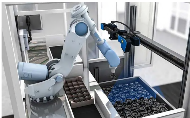
Fig. 3: Process of bin-picking, [47]
