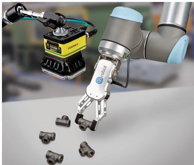
Fig. 4: Bin-picking with 2D camera, [52]
