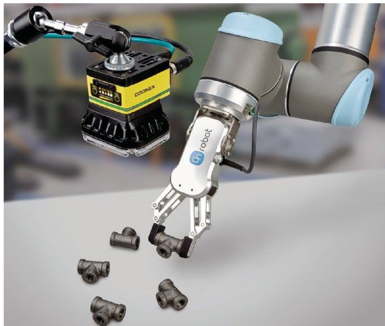
Fig. 4: Bin-picking with 2D camera, [52]
