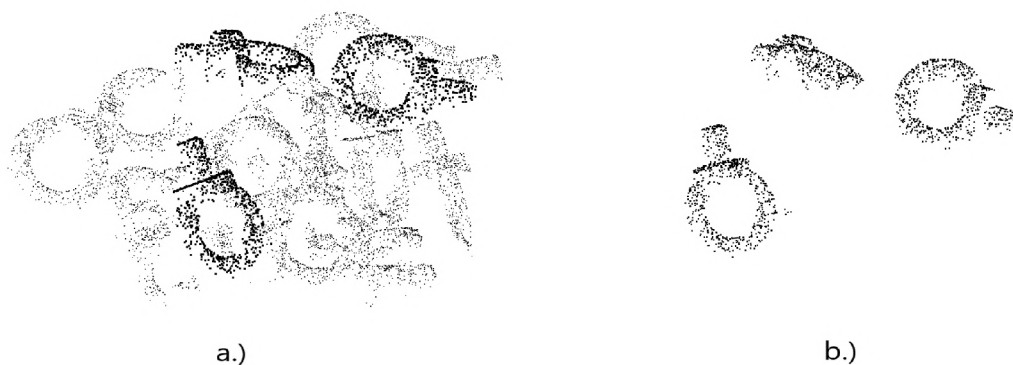
Fig. 64: Ring screw Registration : a.) Highlighted segments. b.) Isolated segments
