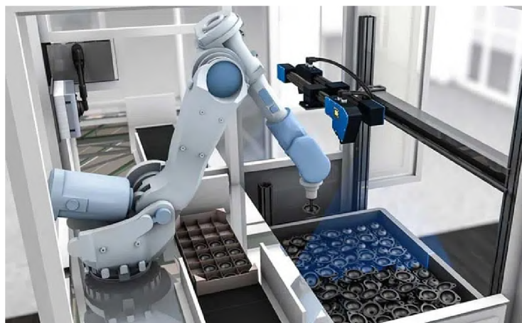
Fig. 3: Process of bin-picking, [47]
