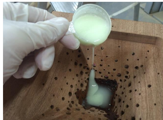
Fig. 106: Holes poured by resin
