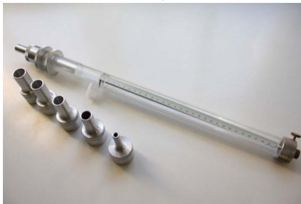
Figure 24. Model of the subglottal tract ready to use (top – mounting of the tract and its position in the table; bottom – the assembled tract and the adaptors for different tracheal diameters).
