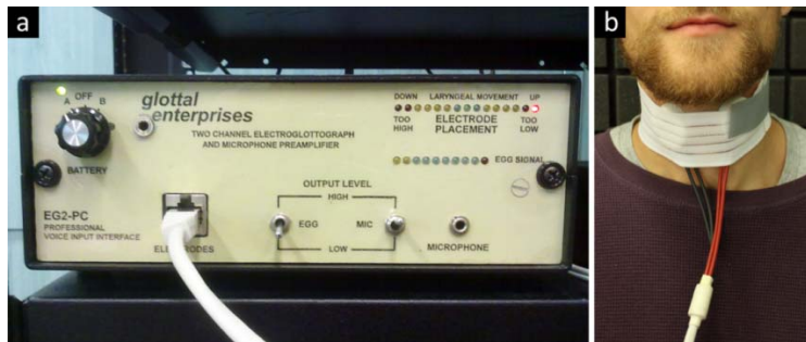
Figure 17. Front panel of EGG device (a) and electrodes attached to the neck (b).
