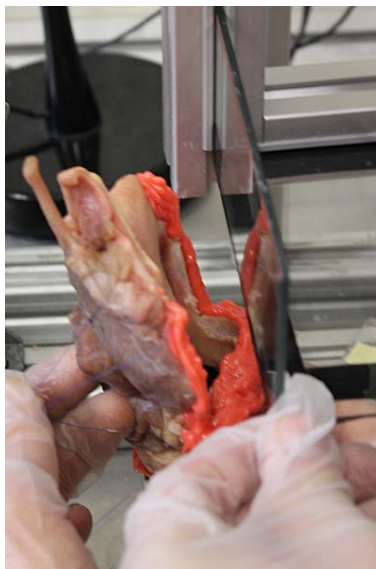
Figure 28. The L-shaped mortise covered with Dental cement (red) for sticking the hemilarynx onto the glass plates.
