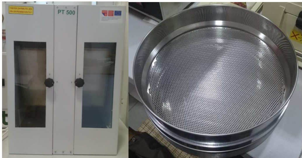
Figure 15. Durability tester for pellets with sieve (Source: Author, 2017)
