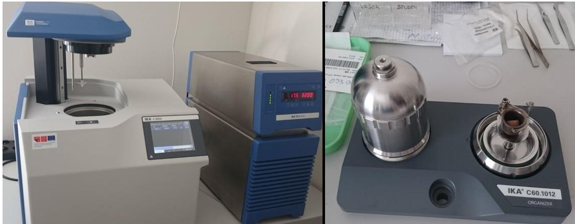
Figure 8. Calorimeter IKA 6000 and prepared pellet in oxygen bomb (Source: Author, 2016)
