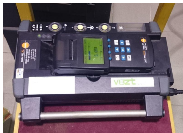
Figure 17. Emission analyzer Testo 350 XL (Source: Author, 2017)
