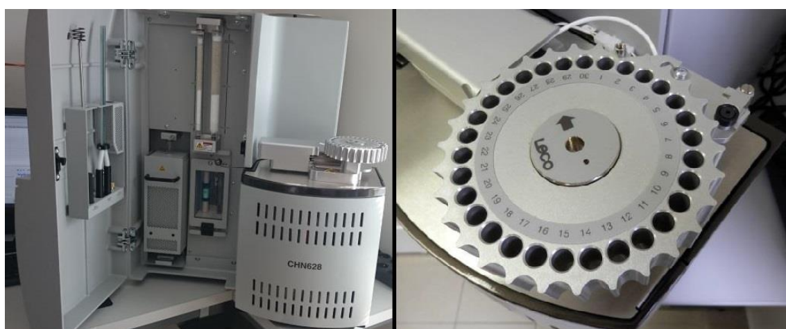
Figure 7. LECO CHN628 Determinator with autoloader (Source: Author, 2016)
