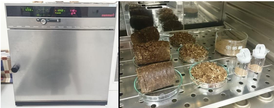
Figure 13. Oven Memmert 100-800 and prepared samples (Source: Author, 2016)
