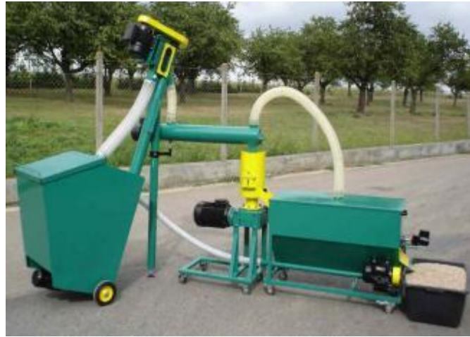
Figure 11. Pelleting line MGL 200 (Source: Kovo Novák, 2016)
