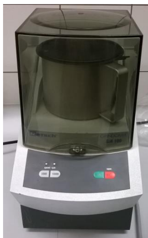
Figure 5. Grinding knife mill Retsch Grindomix GM 100 (Vlachosová, 2016).
