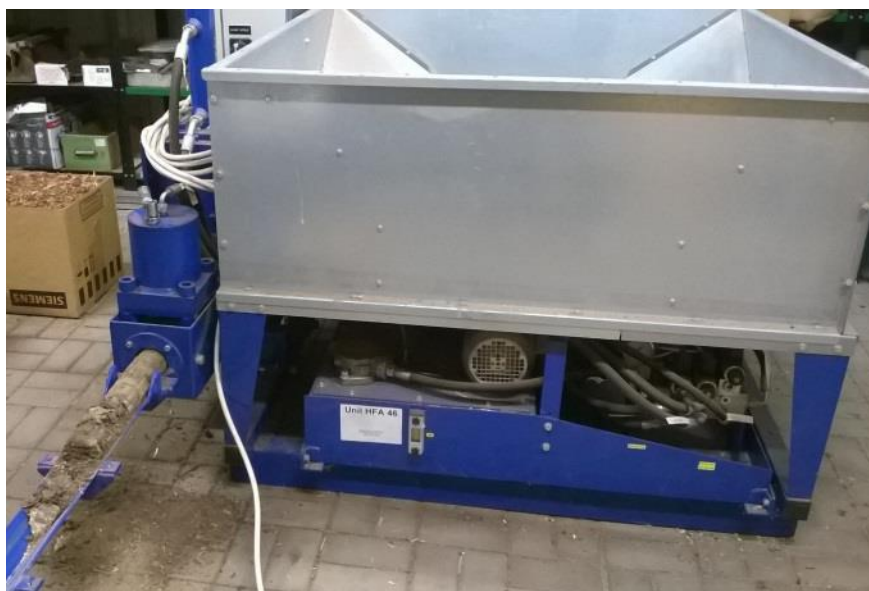
Figure 10. Hydraulic piston press Brikstar (Source: Vlachosová, 2016).
