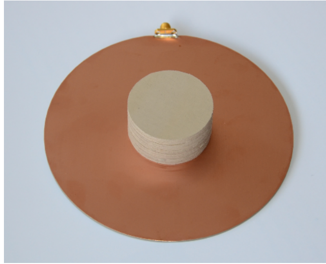
Fig. 3.28: Manufactured prototype of the high gain cylindrical DRA
