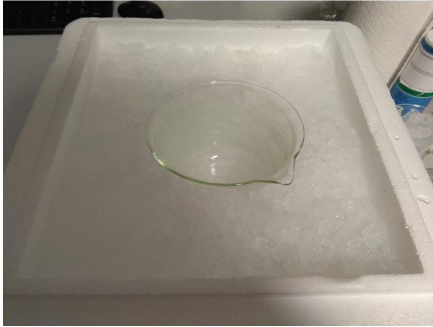
Figure 12: Box filled with ice containing a beaker for petri dish with sample.
