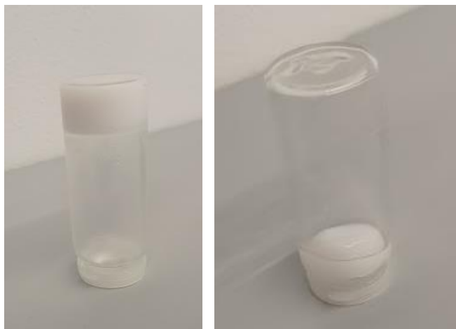
Fig 5.2. Inverted tube with ( on the left ) sample in gel phase and ( on the right ) sample after 10 minutes and the onset of flow.
