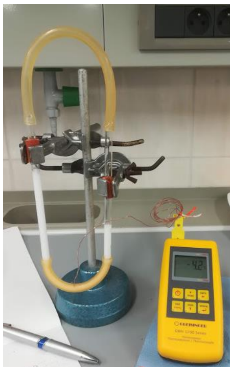
Fig. 4.4. U-shaped tube experimental set-up. Where the limbs are glass tubes of constant diameter, the bottom is a silicone section containing a K-type thermometer probe and on the top there is a silicone sealing.
