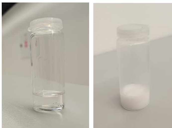
Fig 5.1. On the left, resulting solution of dissolving PCL in AA:FA:At solvent system. On the right, resulting gel from storing the same solution in a freezer for over 45 minutes.
