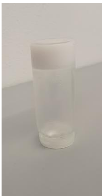
Fig 4.2. Inverted tube with sample in gel phase at the top of the set-up.
