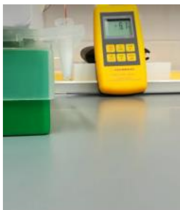
Fig 4.6. Second iteration of the visual experiments using Eppendorf tubes and a K-type thermal probe connected to a thermometer.
