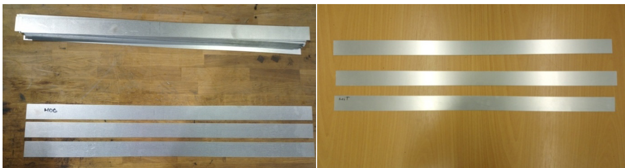
Fig. 5.2 Samples after shearing (HDG– left, NIT - right)
