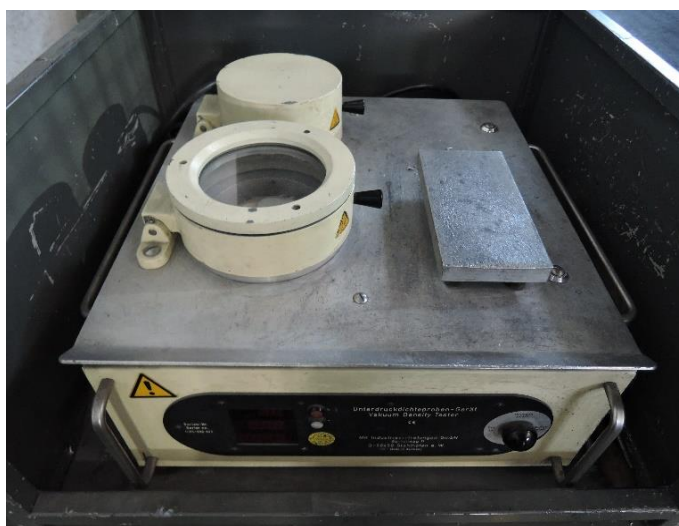
Obr. 9-3 Vacuum density tester, Stahlhofen
