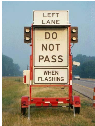
Figure 2.5 Typical dynamic lane merge equipment
