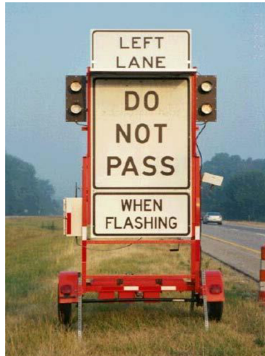
Figure 2.5 Typical dynamic lane merge equipment
