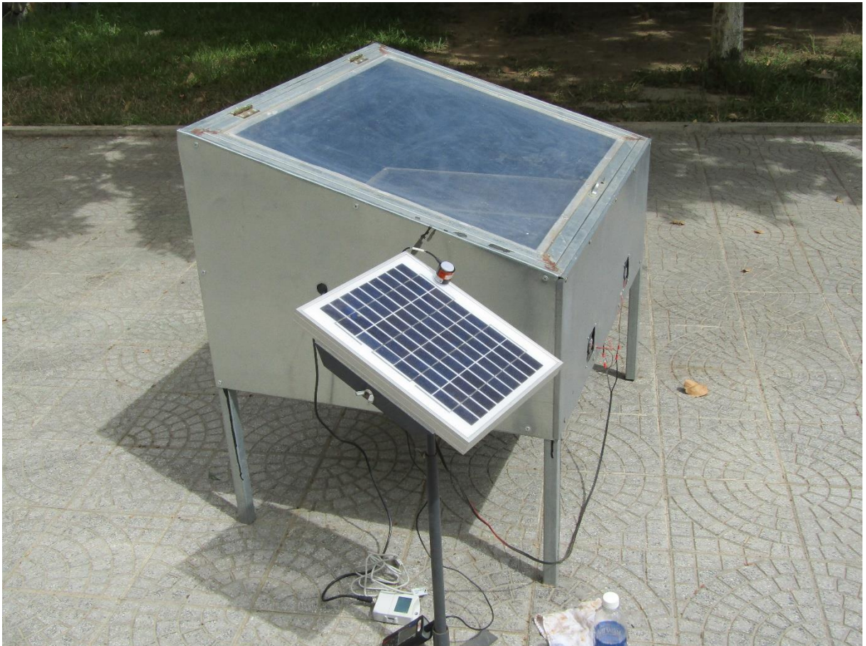
Figure 11. Active solar dryer, which were used in experiment.
