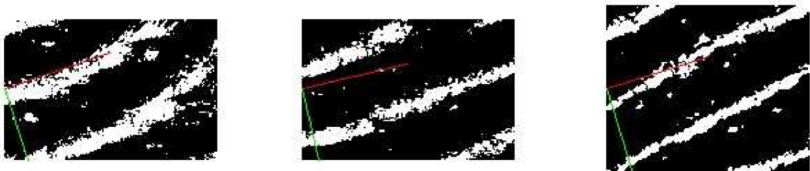
Figure 5.2. Display of direction line (red) and normal line (green) on a sample from several sequences of a live fingerprint images.
