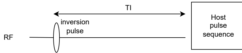
Fig. 2.3: Inversion recovery pulse sequence diagram.
