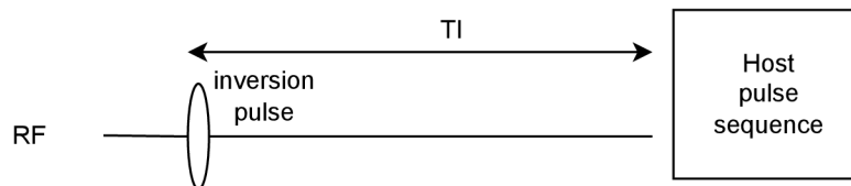
Fig. 2.3: Inversion recovery pulse sequence diagram.
