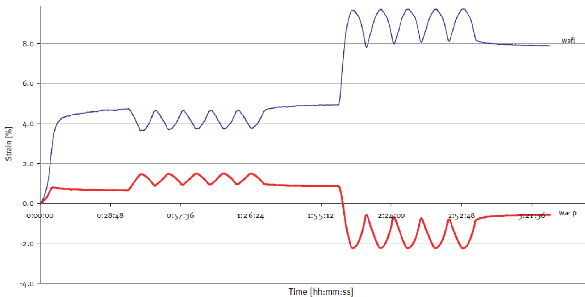
Fig. 150 Biaxial Test: Measured Strains [80]
