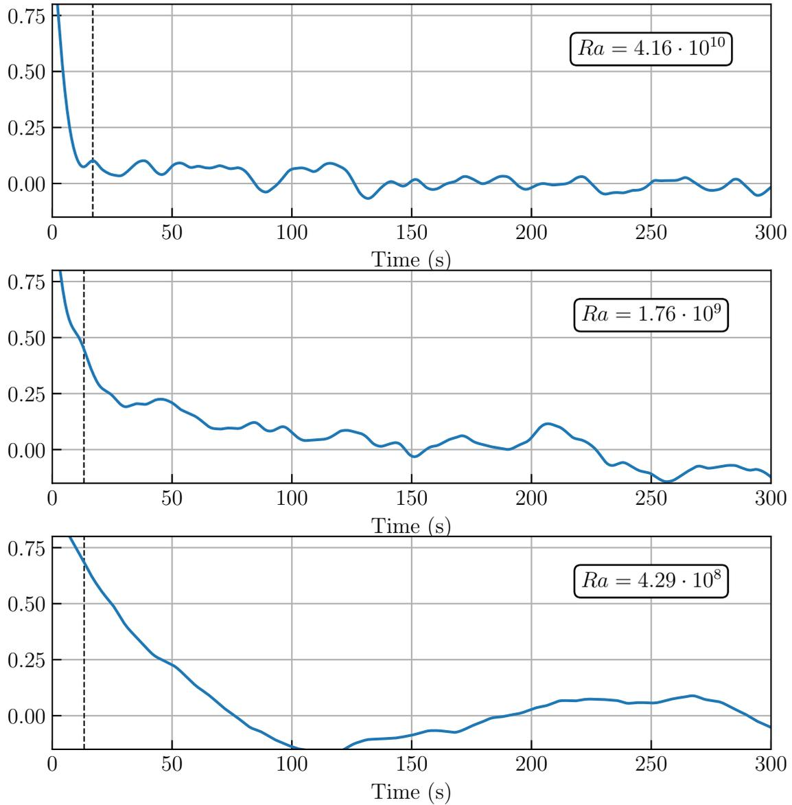
**Figure 4.15:** Auto-correlation functions of the temperature fluctuations of the bottom plate  $T_{b3}$  in CF regime plotted near their central maximum for three different Rayleigh numbers. Position of the first peak in the auto-correlation function of temperature recorded at the bulk sensor is represented by a dashed line.
