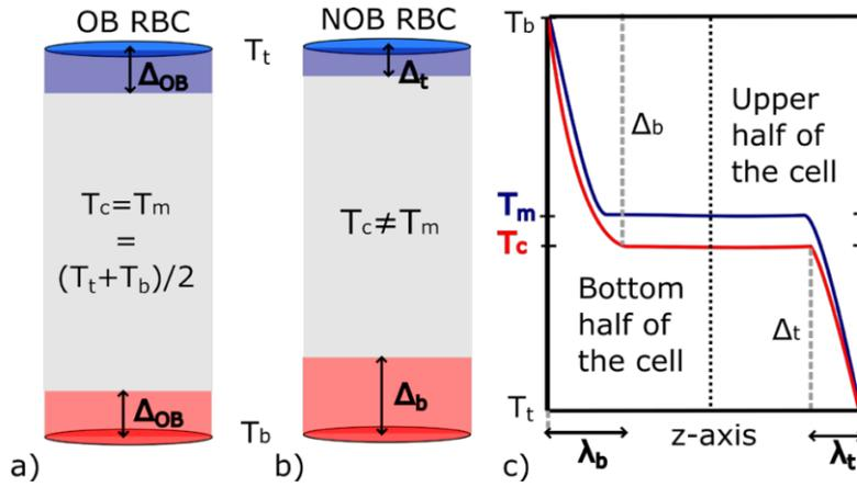
**Figure 1.3:** Scheme of the asymmetry in thermal boundary layers occurring in the RBC due to non-Oberbeck-Boussinesq effects.  $\Delta_{OB}$  is the temperature difference at thermal boundary layers in the Oberbeck-Boussinesq case and  $\Delta_t$  and  $\Delta_b$  are temperature differences at top and bottom thermal boundary layer in the non-Oberbeck-Boussinesq case. Taken from [22].
