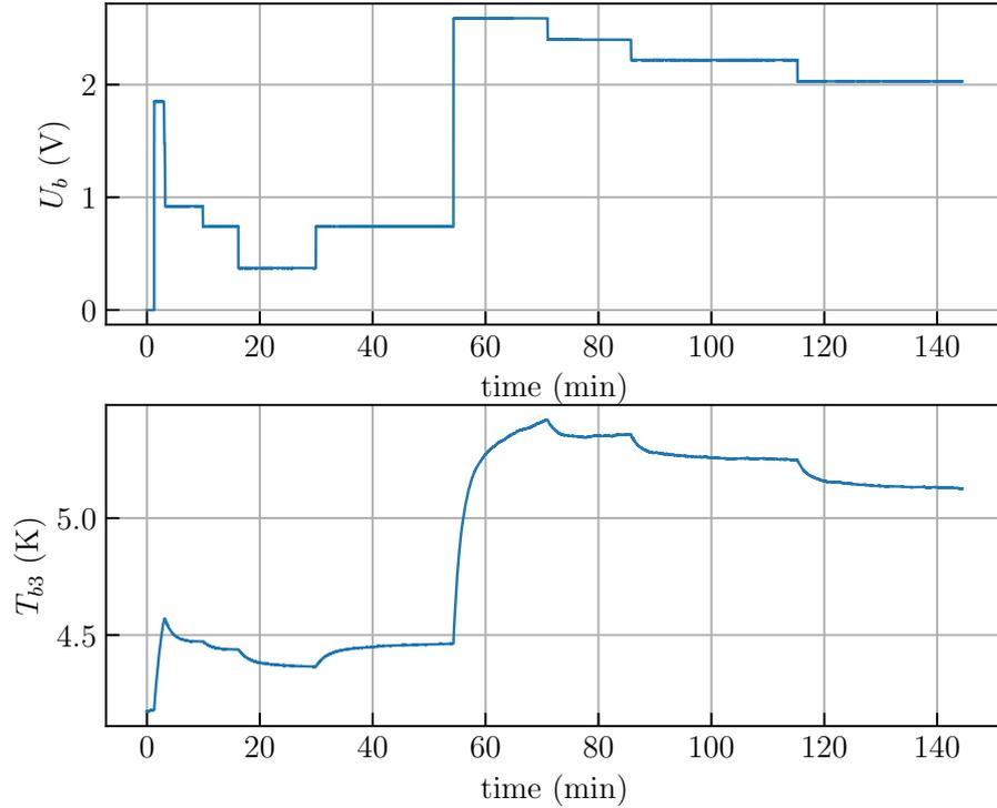
**Figure 3.5:** To get characteristic parameters  $K_p$ ,  $\tau_p$  and  $\theta$  needed for the PID tuning, the step-test was performed. In the upper panel, the input voltage  $U_b$  into the bottom heater is recorded. In the lower panel, for every step change in the input voltage  $U_b$ , there is a corresponding temperature change of the bottom plate  $T_{b3}$  measured by fast Si diode.
