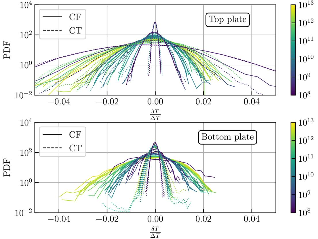
**Figure 4.10:** Calculated probability density functions for all our measurements. For the bottom plate case, a clear distinction between CF and CT regime is visible. In the CF regime, the range of the temperature fluctuations is growing with rising  $Ra$ . The same trend can be seen for the CT regime but the dependence is much weaker. In contrast, the top plate probability density functions for the CT regime are mixed with the CF regime.
