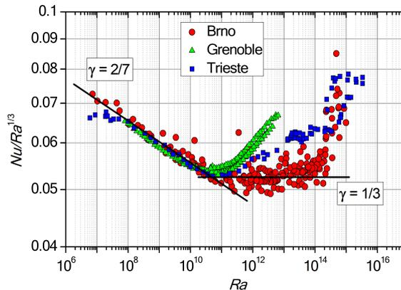
**Figure 2.1:** Experimental dependence of reduced Nusselt number  $Nu$  on Rayleigh number  $Ra$  in experimental cell of aspect ratio  $\Gamma = 1$  from three different laboratories. Data are side-walls corrected. Up to  $Ra \approx 10^{11}$ , they all follow scaling  $\gamma = 2/7$ . For  $Ra > 10^{11}$ , they all start to disagree mutually. Taken from [28].
