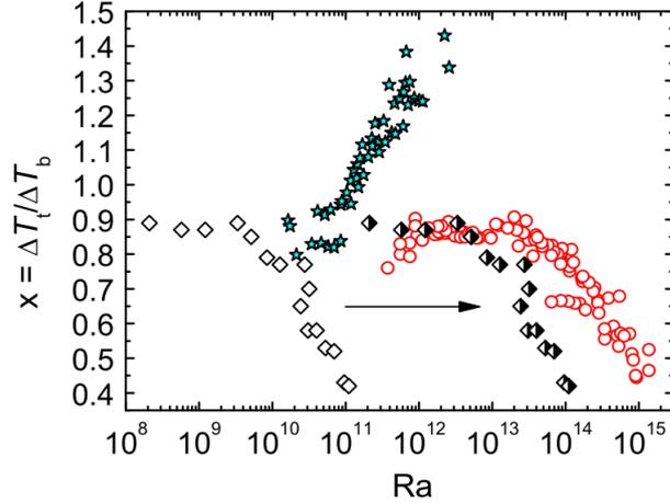
**Figure 1.5:**  $X$  parameter defined in 1.13 measured by different laboratories and for different working fluids where you can see  $X$  parameter rise for the water data (stars) and drop for He data (diamonds and circles). Half filled diamonds are corrected empty diamonds. Circles are data from Brno [4].
