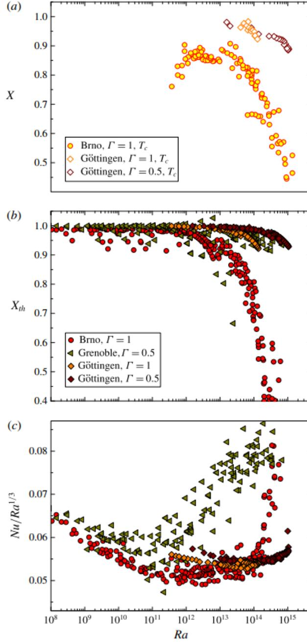
**Figure 1.4:** (a):  $Ra$  dependence of  $X$  parameter calculated from directly measured temperature of the bulk  $T_c$  on  $Ra$ . (b): Calculated theoretical parameter  $X_{th}$  from the fluid properties. (c):  $Nu(Ra)$  dependence where there is clear correlation between decrease in  $X$  parameter and increase in  $Nu$  for Brno measurements. Taken from [18].
