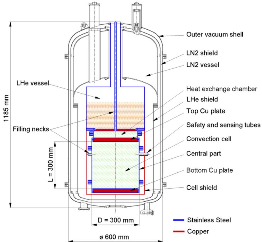
**Figure 3.1:** The helium cryostat with the cylindrical experimental cell used for our measurements [30].
