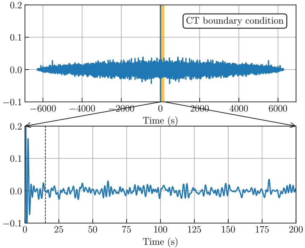
**Figure 4.14:** Auto-correlation function of the temperature fluctuations  $T_{b3}$  on the bottom plate at constant temperature (CT) boundary condition. The noisy behavior of the signal prevents any clear determination of the characteristic time of the large scale circulation  $t_0$ . Measured at  $Ra \approx 1.9 \cdot 10^{12}$ . Position of the first peak in the auto-correlation function of temperature recorded at the bulk sensor is represented by a dashed line.
