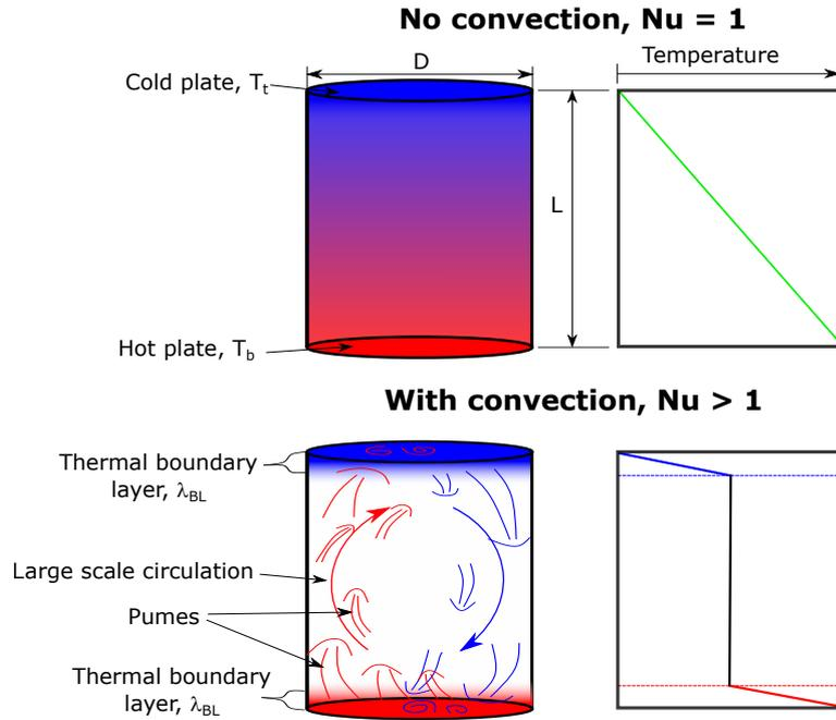
**Figure 1.2:** In the upper panel, the heat inside the cell is transferred just by conduction which is manifested in the linear temperature profile. The basic scheme of the Rayleigh-Bénard convection is in the lower panel. Whole temperature difference  $\Delta T = T_b - T_t$  occurs on two thermal boundary layers of thickness  $\lambda_{BL}$  where the heat is transferred by conduction. In the bulk, the fluid is effectively mixed resulting in approximately constant temperature.
