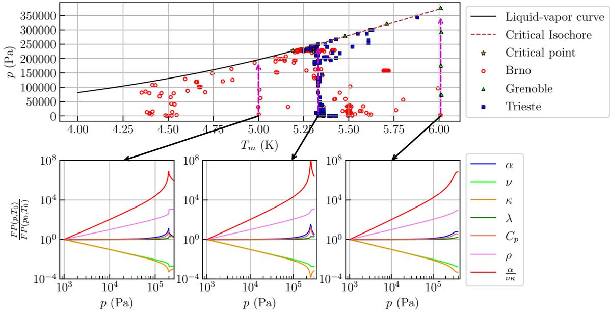
**Figure 2.2:** In the upper panel, phase diagram of helium with Grenoble and Trieste data is displayed. In the lower panel, relative fluid properties along the red arrows are evaluated.  $p_0 = 1000$  Pa and  $T_0$  is 5.010, 5.330 and 6.009 K for respectively.
