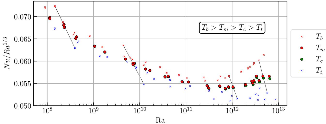
**Figure 4.7:** Reduced Nusselt number  $Nu$  on Rayleigh number  $Ra$  for our Brno measurements where all fluid properties are calculated from temperature of the bottom plate  $T_b$ , top plate  $T_t$ , mean temperature  $T_m$  and bulk temperature  $T_c$ . Connecting black lines are for better orientation in the graph because non-Oberbeck-Boussinesq effects cause the shift in  $Nu$  and also in  $Ra$  and thus mixing the points.
