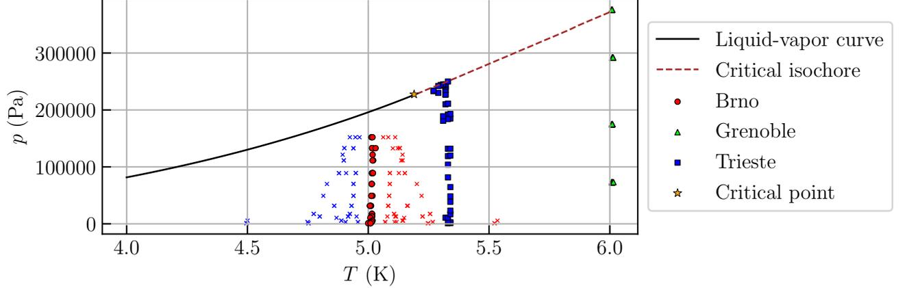
**Figure 4.1:**  $p$ - $T$  phase diagram of the helium with marked helium states at  $T_m$  in our Brno measurements displayed by red circles together with temperatures of the top and bottom plate represented by crosses. Working points used in Grenoble and Trieste experiments are displayed as well.
