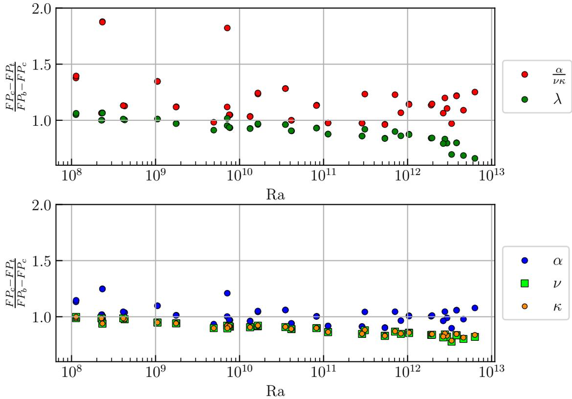
**Figure 4.5:** Behavior of the  $\alpha\Delta T$  can be clearly seen in the behavior of the ratio  $\alpha/\nu\kappa$ , just with the reversed sign. Other properties are nearly one meaning the most Oberbeck-Boussinesq case. Thermal conductivity of the fluid  $\lambda$  follows a rise for  $Ra > 10^{12}$ .
