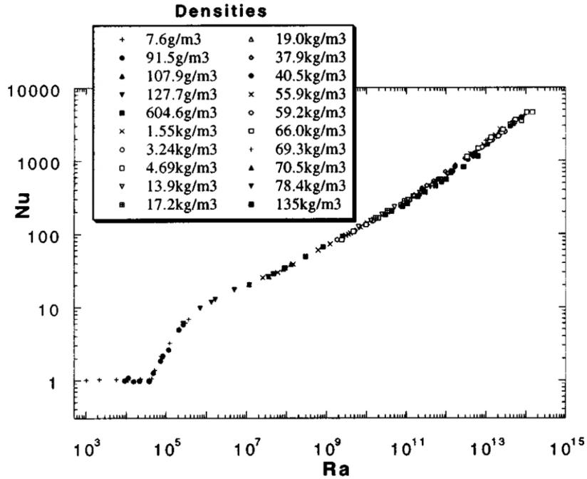
**Figure 1.1:** Experimental dependence of Nusselt number  $Nu$  on  $Ra$  measured with cryogenic helium gas.  $Nu = 1$  means no convection, the temperature profile inside the experimental cell is linear as is displayed in figure 1.2. Then the efficiency of heat transfer is getting higher due to convective heat transfer. Figure taken from [14].
