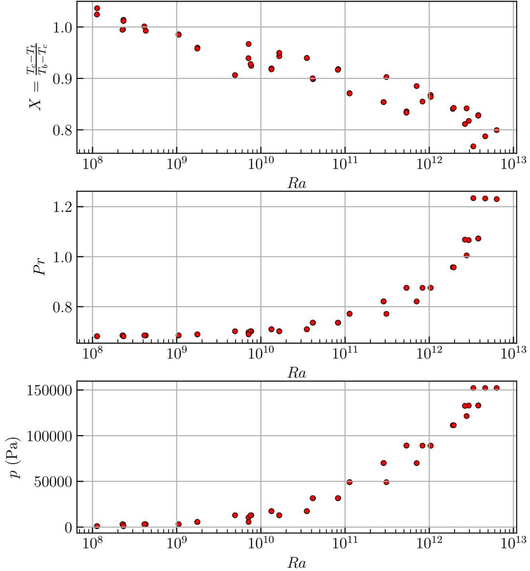
**Figure 4.3:** Top panel:  $X$  parameter defined in 1.13 and also presented in figure 1.5 measured in our Brno experiment. Middle panel: Prandtl numbers  $Pr$  evaluated for every measurement. Bottom panel: Pressure  $p$  inside the experimental cell.
