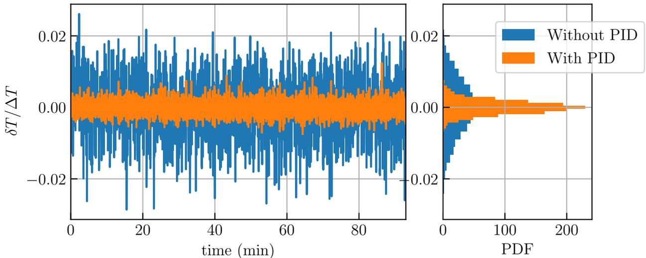
**Figure 4.9:** Record of the temperature fluctuations measured on the bottom plate with (CT regime) and without PID (CF regime). Also their corresponding probability density functions are displayed. Clear narrowing is visible.
