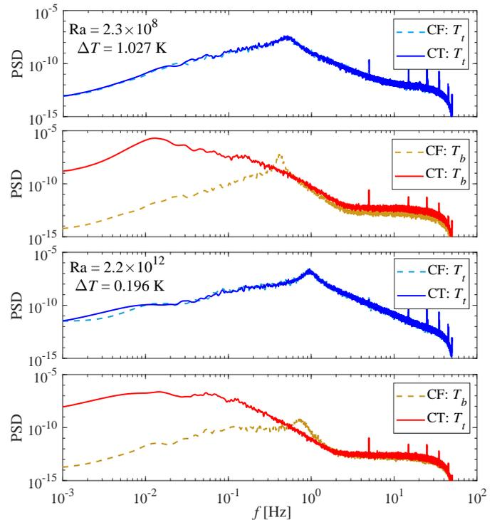
Fig. 3: PSDs of the fluctuating temperature calculated for the cases shown in Fig. 2 display significant depletion at frequencies below 0.4 Hz (0.7 Hz) for the lower (higher) Ra cases; faster temperature fluctuations of the bottom plate are hardly affected by the PID control (red lines). At the top plate, PSDs (blue lines) remain entirely unaffected at all measured Ra.
