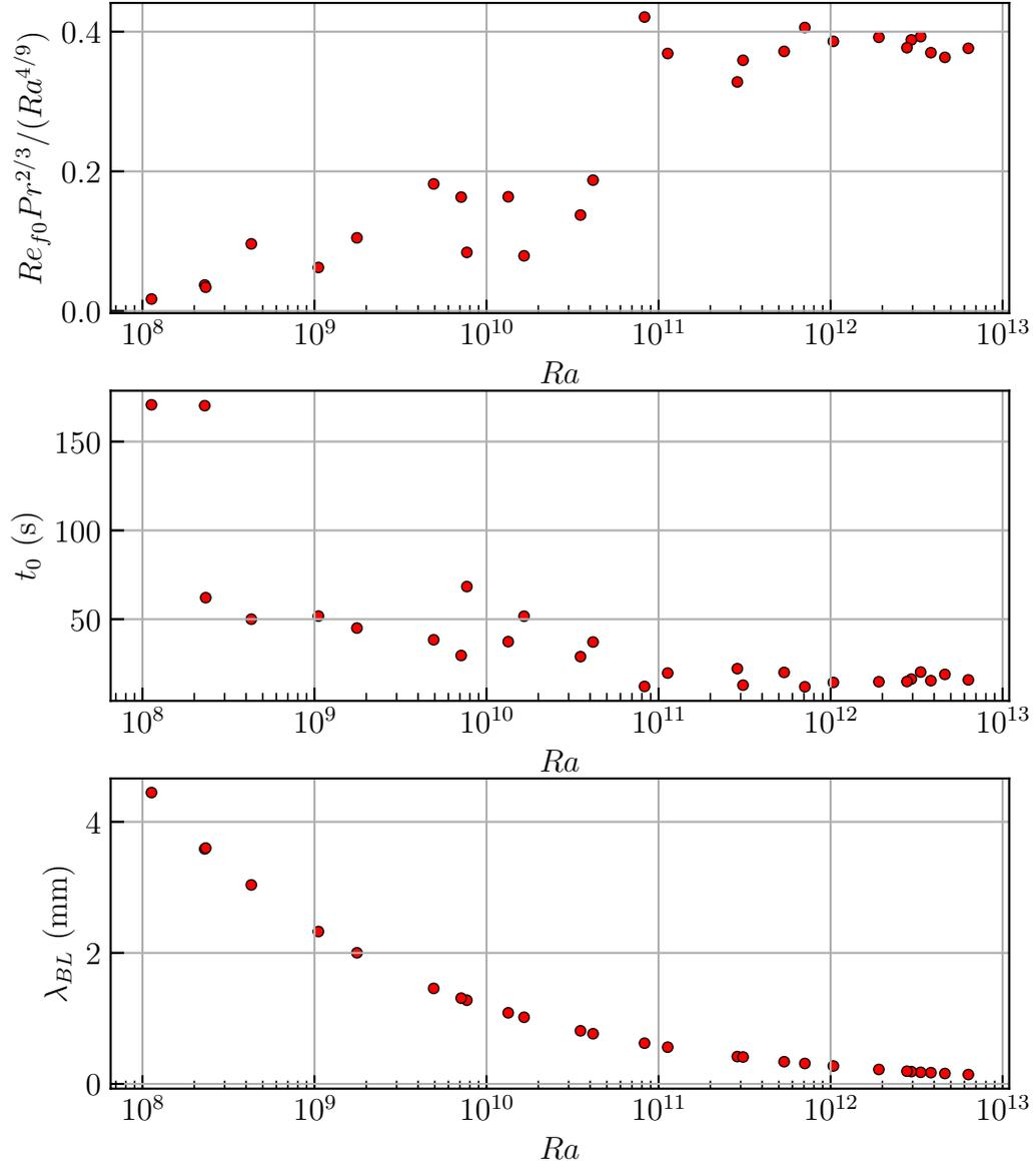
**Figure 4.16:** Approximate evaluation of the reduced Reynolds number  $Re_{f_0}$  obtained from the equation 1.15 [25].  $t_0$  was estimated from the first visible peak of the auto-correlation functions of the temperature signal of the bottom plate. In the bottom panel, thickness of the thermal boundary layer  $\lambda_{BL}$  is evaluated.
