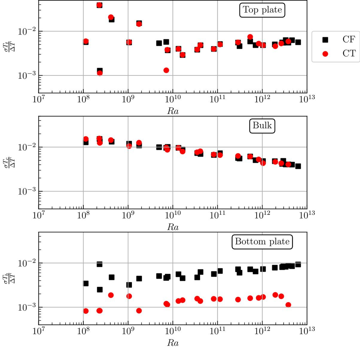
**Figure 4.11:** Calculated normalized standard deviations of the temperature fluctuations of the bottom plate, top plate and also temperature fluctuations of the bulk  $T_c$ . The increasing trend with increasing  $Ra$  for the bottom plate is obvious. A clear decrease is visible for the temperature fluctuations in the bulk with growing  $Ra$ .
