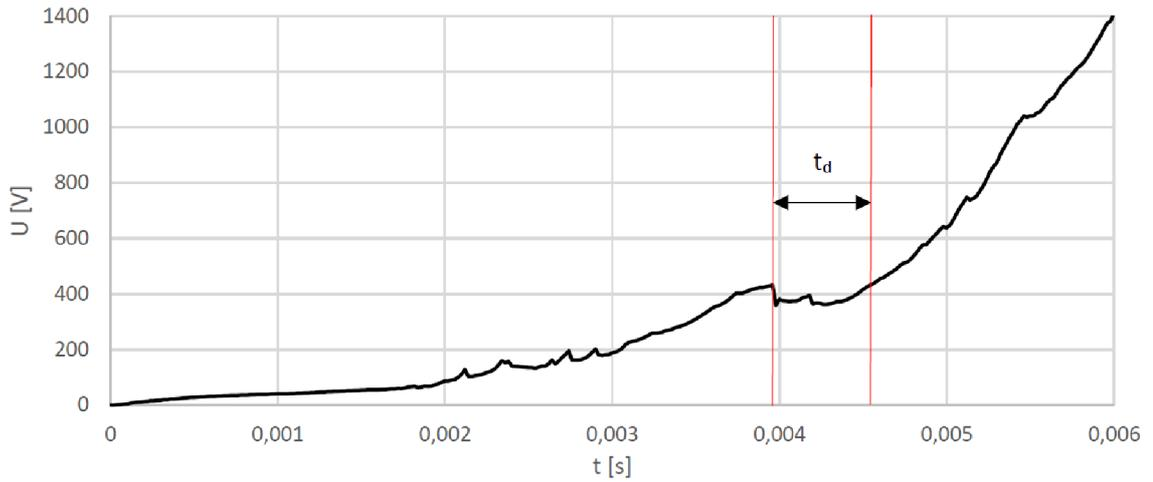
Fig. 9.1: Back-commutation delay
