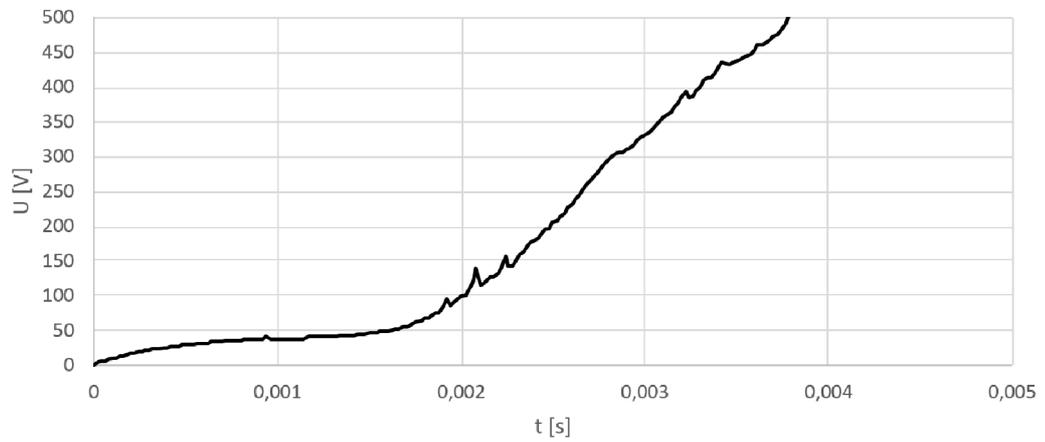
Fig. 9.3: Arc voltage - AR2-03;AR1-01;PP-02
