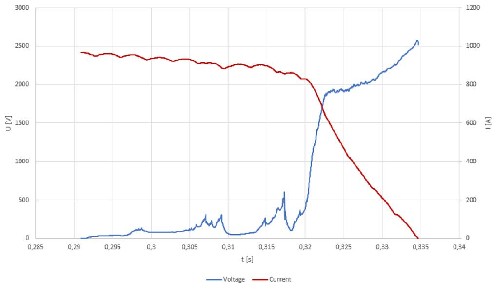
Fig. 4.2: Breaking operation voltage waveform - contactor
