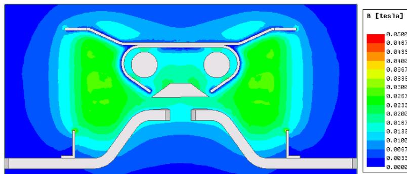
Fig. 1.3: Magnetic field distribution with steel arc runners
