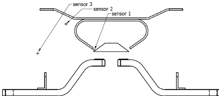
Fig. 5.2: Pressure sensor placement
