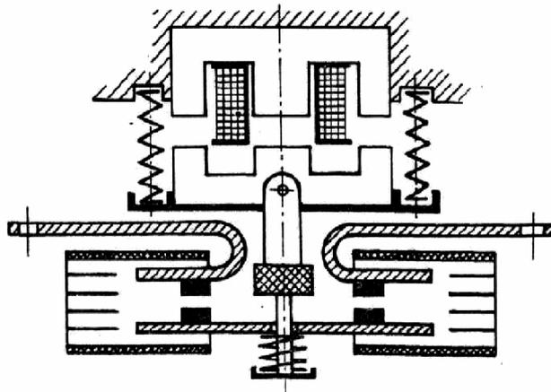
Fig. 1.1: Basic contactor construction [1]
