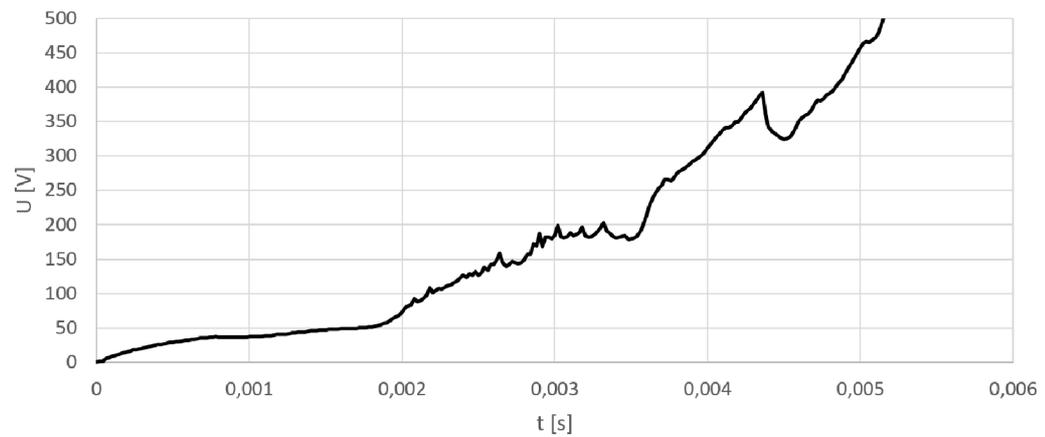
Fig. 9.4: Arc voltage - AR2-03;AR1-01
