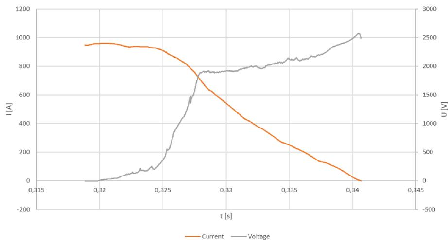
Fig. 5.8: Arc voltage and current waveforms
