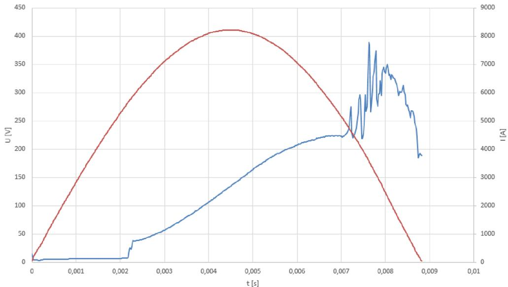
Fig. 4.1: Breaking operation voltage waveform - MCCB
