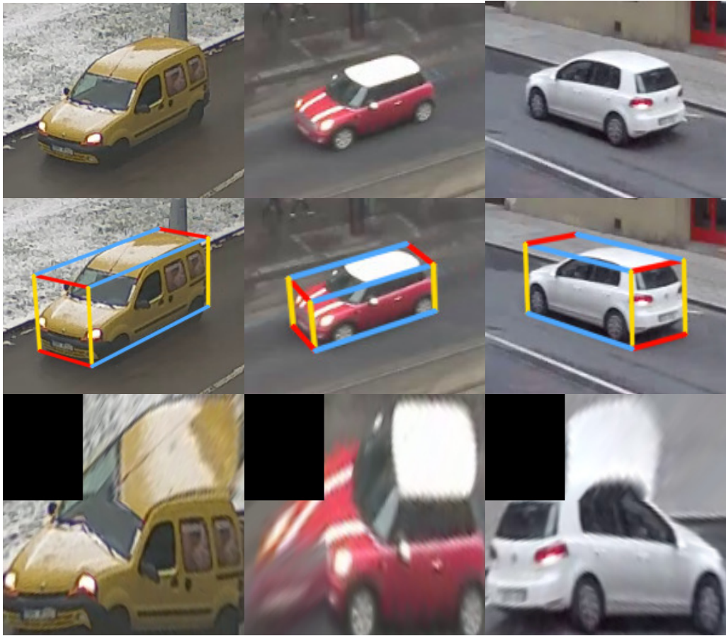
Figure 4.2: Examples of vehicles (top), their 3D bounding boxes (middle) and unpacked version of the vehicles (bottom).
