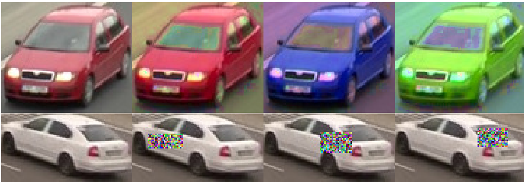
Figure 5.5: Examples of proposed data augmentation techniques. Left most image contains the original cropped image of the vehicle and other images contains augmented versions of the image ( Top – Color , Bottom – ImageDrop ).
