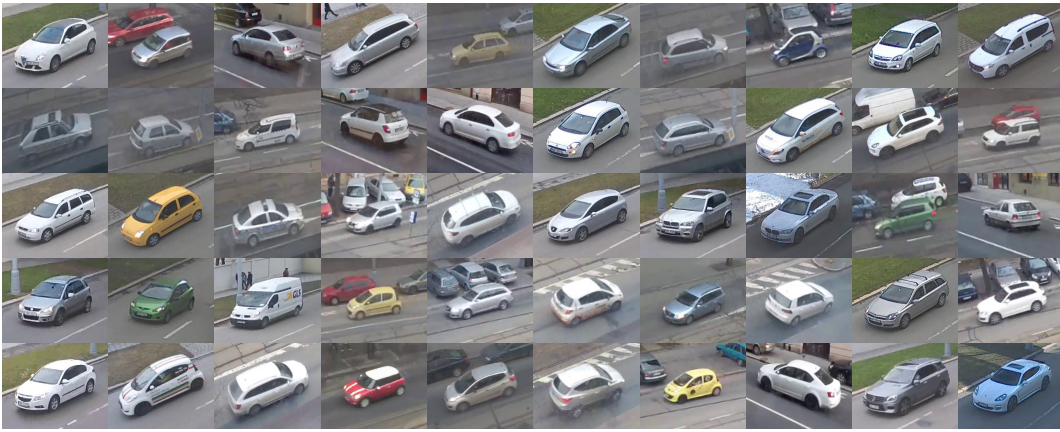
Figure 4.6: A sample of the novel BoxCars dataset. In total, it captures 21,250 vehicles in 63,750 images, from 27 different makes (148 fine-grained classes).
