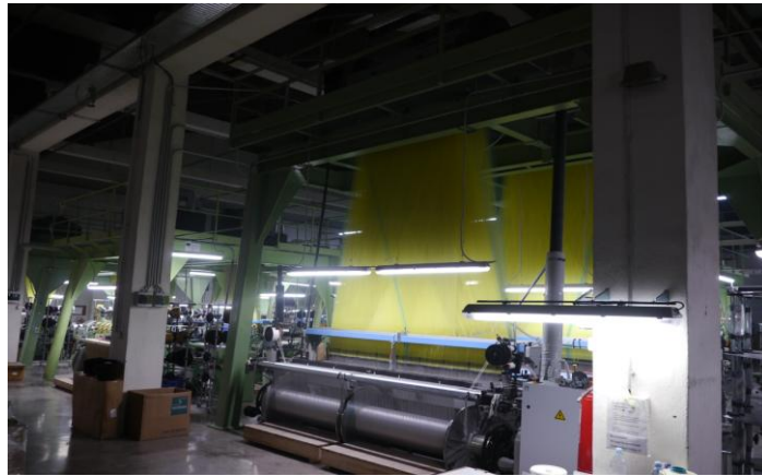
Figure 8: Overall view of the ITEMA weaving machine (Source: Own work)
