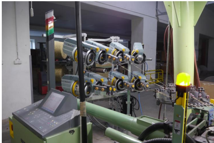
Figure 12: Machine control panel including a monitor and weft dispensers (Source: own work)
