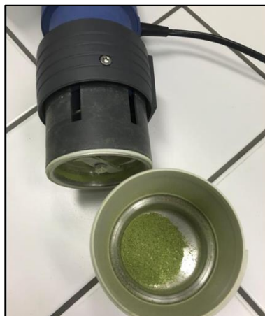
Figure 20 The biomass was milled using IKA A11 basic analytical mill
