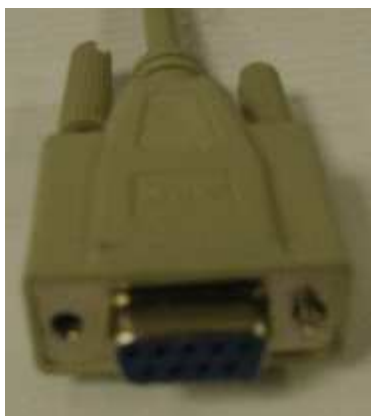
Obr. 2 Konektor RS232 s 9 piny.
