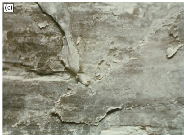
Figure 5 Detail of adhesive wear on engine bearing (AlSn20Cu1 alloy) [32]
