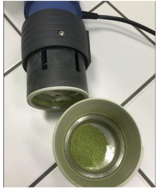
Picture 18 The biomass was ground using an IKA A11 basic analytical mill.
