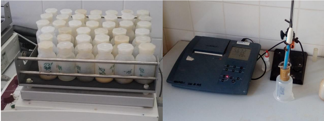
Fig. 9 Soil reaction – Flasks with soil samples in the shaker (left), (Karas, 2015a)
