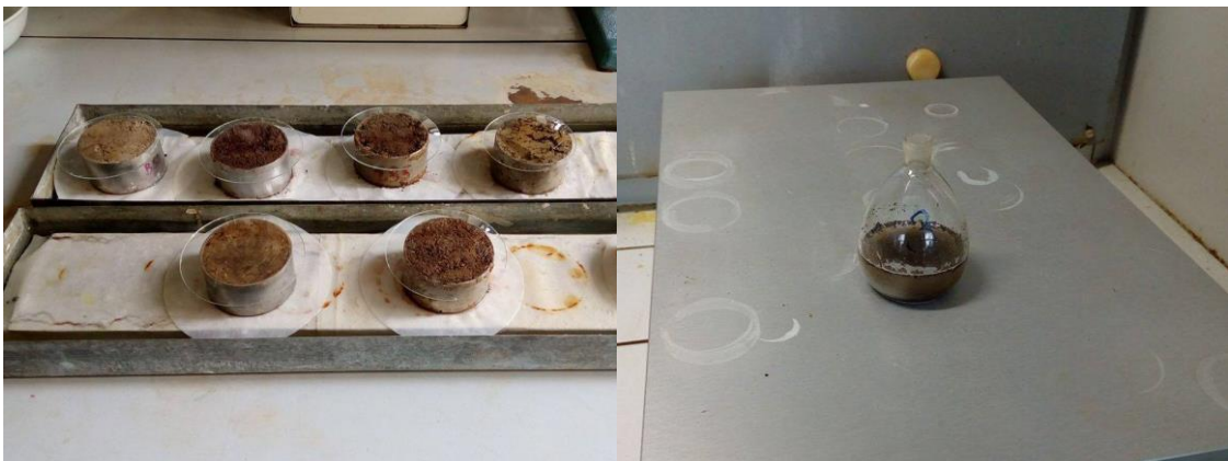
Fig. 11 Maximal capillary water capacity - Kopecky's soil sample ring saturating (left) (Karas, 2015b)
