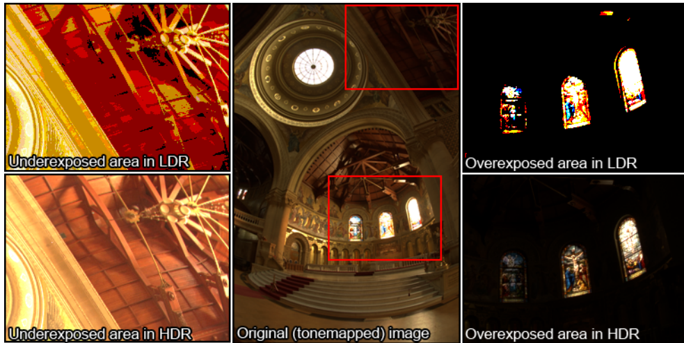
Img. 2.2 - Information content and quantisation errors in HDR and LDR images (based on data from [45], image courtesy of Paul Debevec [13])
