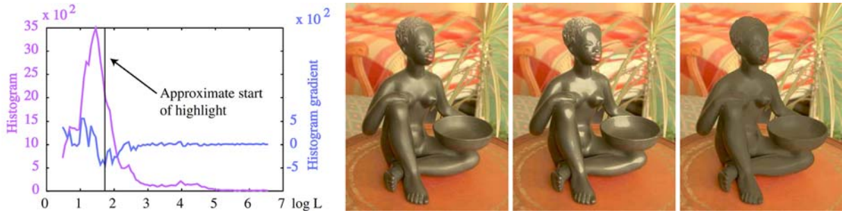
Img. 4.3 - An illustration of the highlight reduction / enhancement algorithm[29] (left – histogram of an HDR image and its derivative, with the detected start of highlight, right – images demonstrating the luminance remapping, from left – original image, enhanced specular component, enhanced diffuse component)
