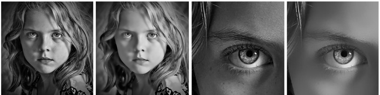
Img. 4.5 - Result of the bilateral filter processing showing the edge-aware blurring effect (for both pairs of the images – left shows the original image and right is the processing result)
