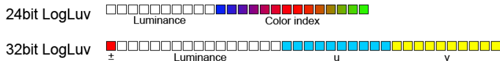
Img. 2.4 - Structure of one pixel in LogLuv version of TIFF file format [45]
