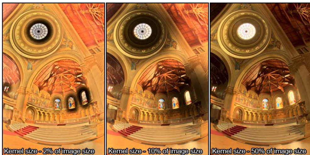
Img. 2.8 - Results of Chiu' operator with different kernel-size parameters (source image courtesy of Paul Debevec [13])
