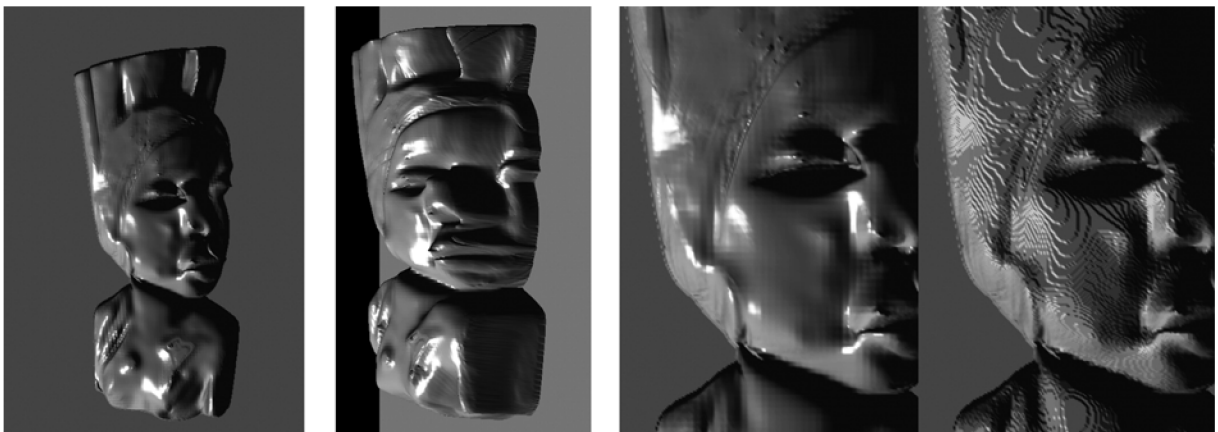
Img. 4.8 - A visualisation of the depth-estimation algorithm results as displayed using OpenGL (left – the extracted shape from the same viewpoint as the source image, middle – a rotated version of the same shape showing only vague correspondence to the original object, right – the effect of the quantisation of the result with non-quantized version on the left side and quantized on the right side)
