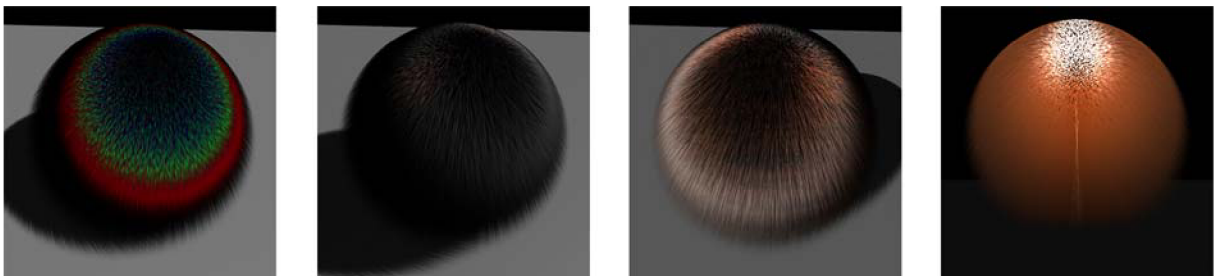
Img. 4.13 - Results of the cross-section scattering model (from left – longitudinal components of the model with N_R in green, N_{TT} in red and N_{TRT} in blue; the fur sphere lit from side; the same sphere lit from front; and the same sphere lit from up behind exposing mainly the TT component)
