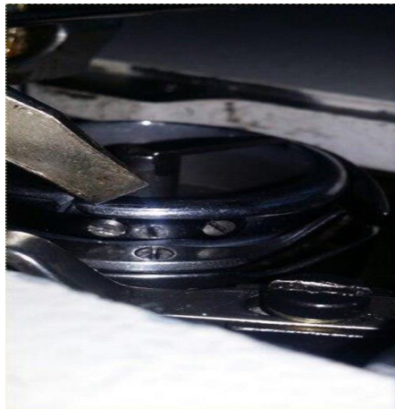
Figure 4. Bobbin thread tension adjustment
