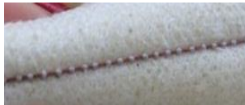
Figure 8. Upper thread pulled towards the bobbin thread
