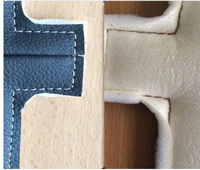
Figure 7. Ideal seam with the binding point in the middle of the seam.
