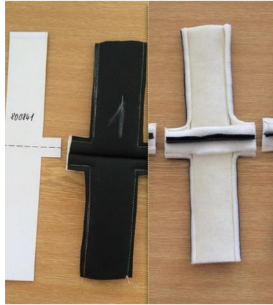
Figure 5. Seams strength testing sample by standard EN ISO 13935
