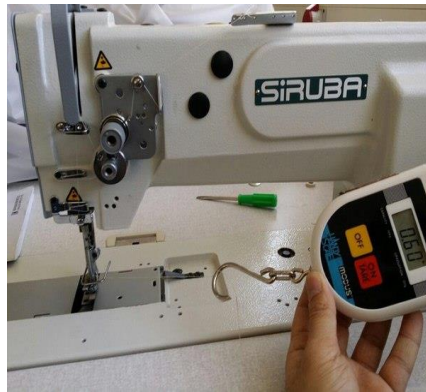
Figure 2. Thread tension measuring device
