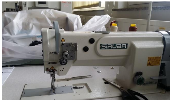
Figure 1. Lockstitch sewing machine used for the experiments
