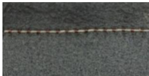
Figure 9. Bobbin thread pulled towards the face of the fabric layer
