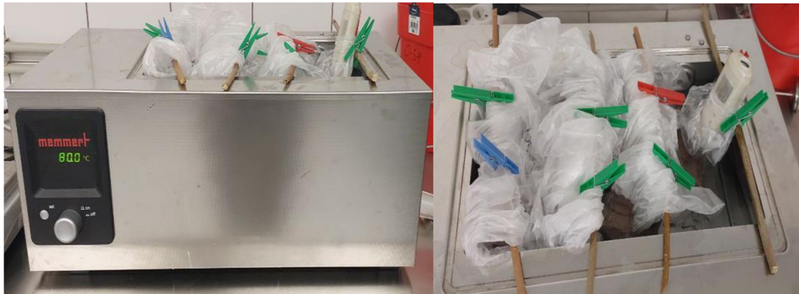
Figure 3 Meat samples were placed in plastic bags, attached to wooden rods, and submerged in a water bath set to 80°C. On the left side of the image, a thermometer is inserted into the meat to monitor and control the cooking temperature.
